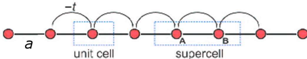
We consider a linear chain of atoms represented by single orbitals, as shown in the figure. The distance between atoms is  $a$ , the tunneling amplitude between nearest neighbors is  $-t$  and we disregard the overlap between neighboring orbitals. It is well known that the electronic states form a cosine band (*Ashcroft & Mermin, Chap. 10*). In this problem you will rederive this simple result. It is recommended that you review the calculation of the band from the Sheet 3, Problem 2.
